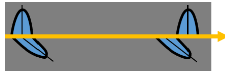
Polarization Mode Dispersion Wavelength polarization modes traveling at different speeds
